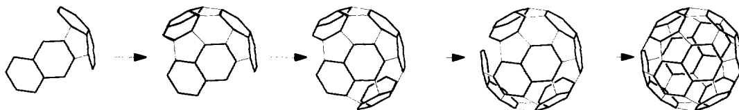
Scheme 1. Six naphthalene-molecules adding to each other and closing to C_{60} (schematically) as proposed by Taylor and Kroto et al. 14-16
